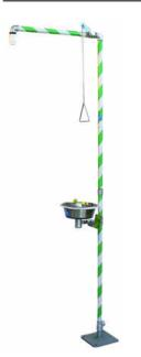
Size Emergency and eye shower MBS150-30 stainless steel (1¼") Article number 999999979 Material Stainless steel bath, Stainless steel pipes, Plastic shower head RVS Pipework Operation Stainless steel push bar and stainless steel pull bar Water flow Shower 80 ltr/min, bath 12 ltr/min. 1<sup>1</sup>/<sub>4</sub>" BSP internal thread Water supply
