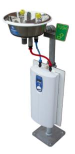
Size Freestanding eye bath with flow-through MB30 ID (Indoor) Article number 999999979 Material Stainless steel eyebath, steel piping Galvanized Pipework Operation Stainless steel push handle Water flow 12 litres/min (2 Bar) 15 mm compression fitting or Water supply 1/2" BSP external thread Water outlet Through the stand pipe Water temp. approx. 25 gr, IP 24 Forwarding
